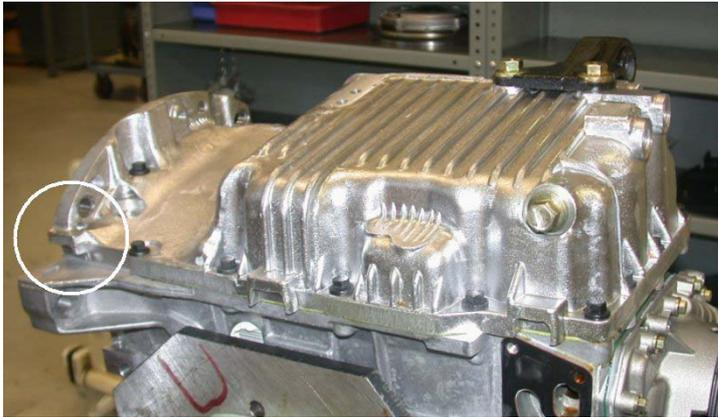
3. Using a suitable steel wedge with an inclusive angle of no more than a 20°, insert between the flange and the ladder (see illustration 2).
