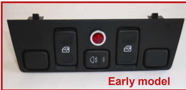
**15** To test water level sensor, switch ignition on. The buzzer will buzz twice and the light will illuminate for a short period. This signifies all is okay. If the light and buzzer continue, then check water level immediately.
