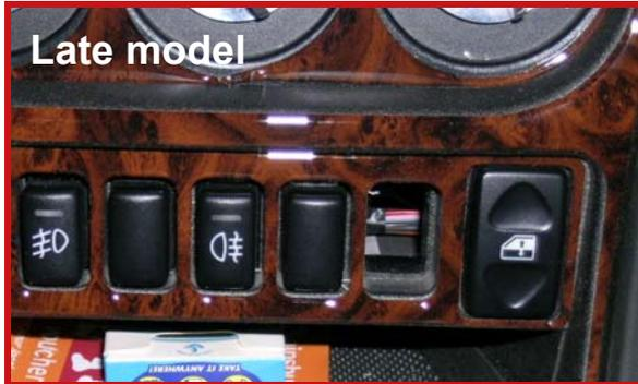
**14** Drill a 7mm hole in a spare switch blank. Alternatively, if you have an early car, drill a hole in the centre of the switch mount. Fit lamp and connect wires.
