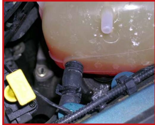
**4** Clip the sensor to the bottom of the new expansion tank and refit in reverse order. Then top up with fluid from the old tank. You may find it necessary to top up with new anti-freeze/water mixture.
